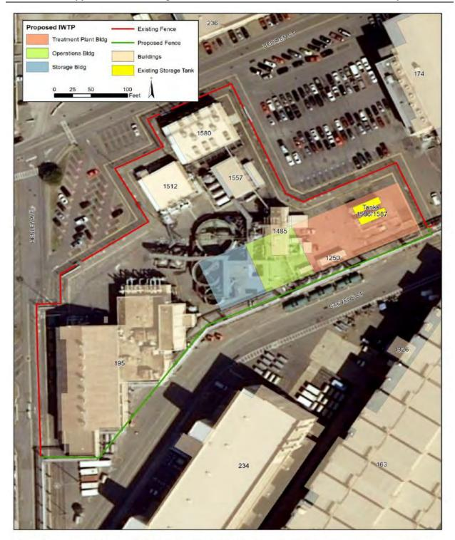
Figure 4: Locations Of The Existing & Proposed Industrial Wastewater Treatment Plant
