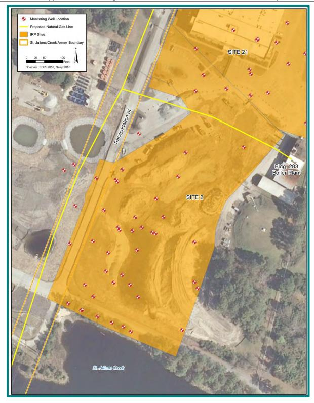
Figure 3.7-2: Location Of Groundwater Monitoring Wells In Installation Restoration Program Sites 2 & 21
