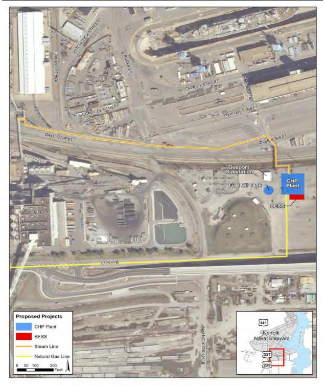
Figure 3: Locations Of The Proposed Combined Heat & Power Plant, & Battery Energy Storage System
