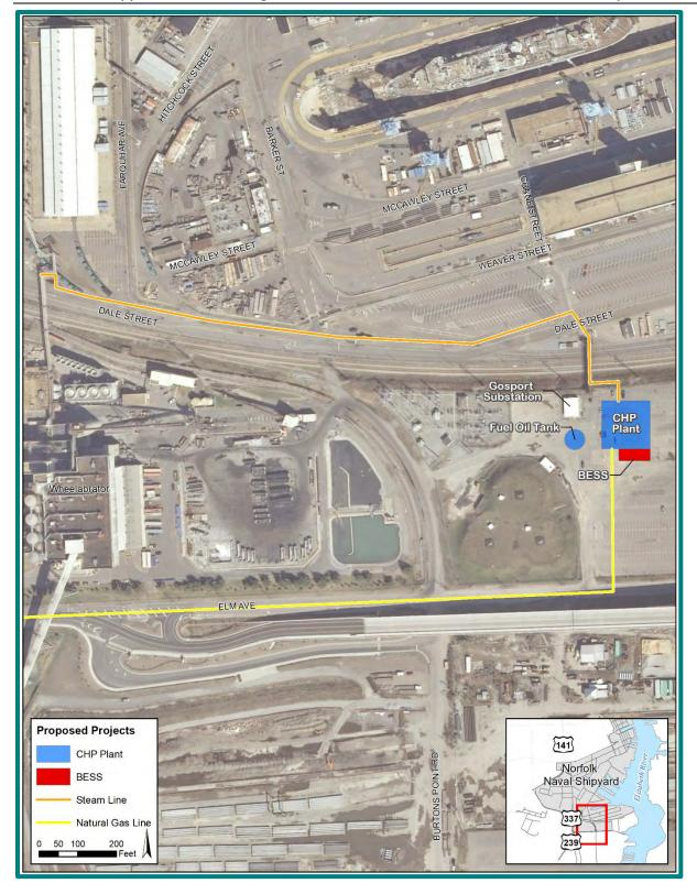
Figure 2.1-3: Location Of The Proposed Combined Heat & Power Plant
